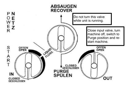
**NOTE:** To change from Recovery mode to Purge: Close the Input port, turn the unit off (to prevent high pressure shutoff), switch to Purge position and restart the unit.
