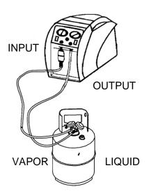
To start you must have a minimum of 2,5 kg of liquid refrigerant in the tank.
